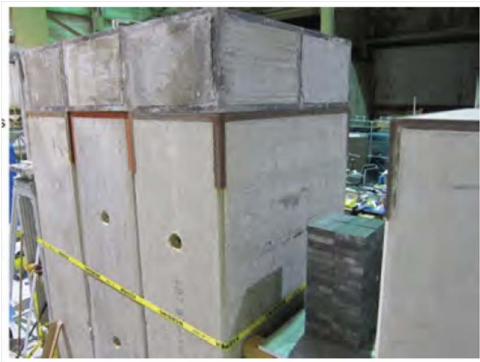
Figure 30 – Experimental drawing of reactor mock-up (top) and photograph (bottom). In the photograph, 2.74 meters of concrete surrounds a stack of lead on each side. The MMT detector planes are oriented on the ends of each slab of concrete (diagramed in orange, top).
