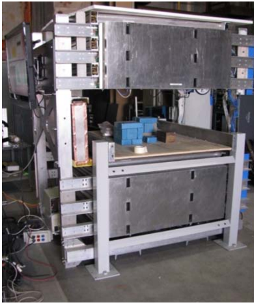
Figure 15 - The mini muon tracker (MMT) in a vertical (standard) orientation. Muon trajectories are measured by drift tubes located in each supermodule. The muon scattering objects in the field of view (e.g., lead blocks seen as blue rectangles in the photo) are reconstructed by the data acquisition computer; their images are displayed on the monitor in real time.
